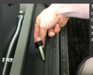
To insure the accuracy of your settings, place the focus tool on top of your material after the z-axis has been adjusted.
